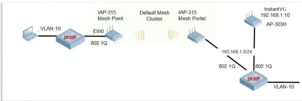
The second one is showing the configuration steps involved in setting manual mesh cluster for a specific Mesh porta/point with E0 bridging.
