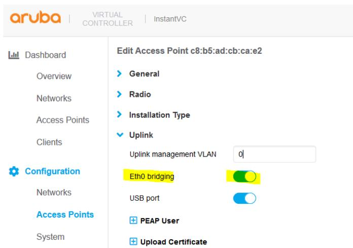
The screenshot shows the 'Edit Access Point' configuration page for the selected IAP 'c8:b5:ad:cb:ca:e2'. The 'Uplink' section is expanded, showing 'Uplink management VLAN' set to '0'. The 'Eth0 bridging' toggle is turned on. Other options like 'USB port', 'PEAP User', and 'Upload Certificate' are visible but not expanded.
