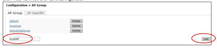
Now select the new "myRAP" AP Group, expand the "Wireless LAN" Profile > "Virtual AP" and use the pull down to add the "myrap-vir" (virtual AP profile) previously created with associated AAA and SSID profiles.
