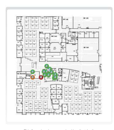
This floor plan shows an unhealthy client (red), which ClientMatch will automatically steer to a better AP and radio to optimize overall performance.
