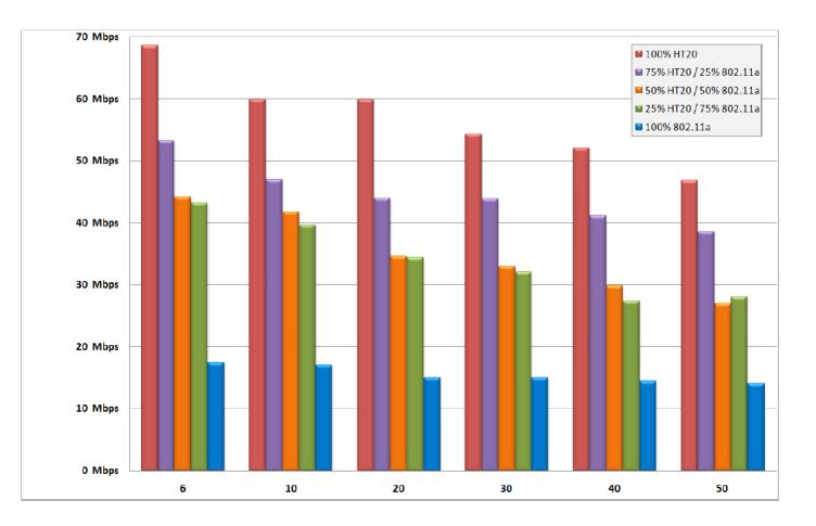
802.11n 5-GHz Aggregate Mixed-Mode TCP Client Scaling Performance (AP-225, HT20, TCP Bidirectional)
