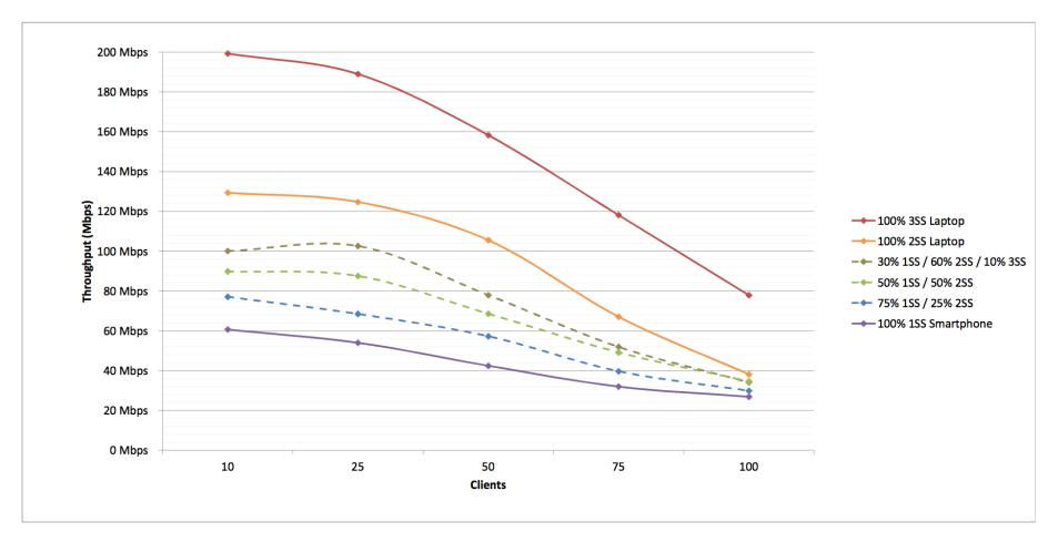
802.11n 5-GHz Aggregate Mixed-Mode TCP Client Scaling Performance (AP-225, VHT20, TCP Bidirectional)
