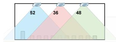
Overhead coverage is a good Choir when uniform signal is desired everywhere in the target area
