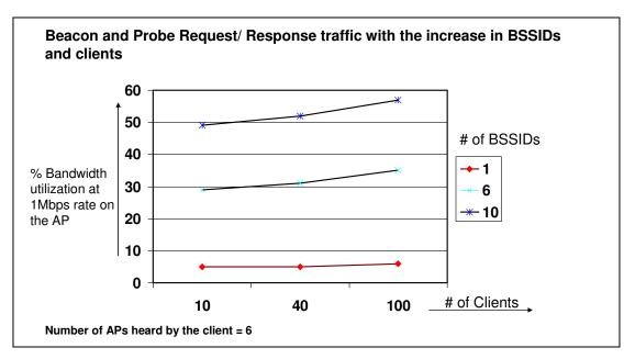
Figure 1.3: The graph shows the effects of multiple virtual AP declarations (1, 6, 10) on 802.11 b/g channel throughput with the
