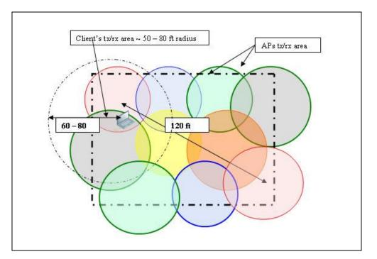
Figure 2.1: 802.11a AP deployment. Note that for the same coverage area (shown in Figure 1) an 802.11a deployment can accommodate more APs on different channels than 802.11b/g greatly reducing the possibilities of the traffic from cells on the same channel bleeding over.
