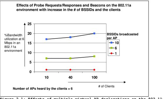
Figure 2.1: Effects of multiple virtual AP declarations on the 802.11a throughput for different number of clients in the APs range.
