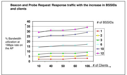
Figure 1.2: Effects of multiple BSSIDs on an 802.11 b/g environment
