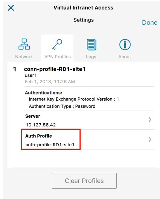
When the authentication fails with one auth-profile, the VIA client switches to another one automatically.
