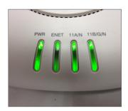
Step 2: Once the front 11A/N or 11B/G/N LED lights turn green,The Instant AP is ready to be set up (about 20-30 seconds)
