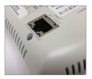
Step 1: Remove Instant AP from packaging and plug-in AC Adapter and Ethernet cable to ENET port
