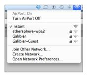
Step 3: Connect to the **instant** SSID once it appears under the Airport Icon (for Mac OSX) or Wireless Network Settings (for Windows).
