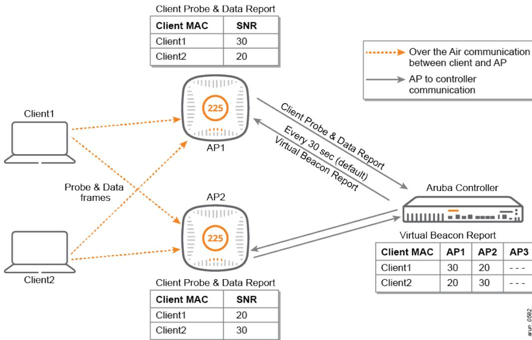
The ClientMatch figure shows how ClientMatch monitors each client's capabilities and connection on a WLAN using probe requests and data frames sent by the client.
