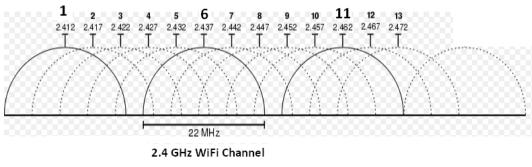
Figure 1: 2.4GHz Channel distribution
