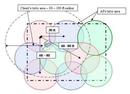
Figure 2: 2.4GHz AP deployment in a given coverage area. Channels used are 1,6,11 (color coded).
