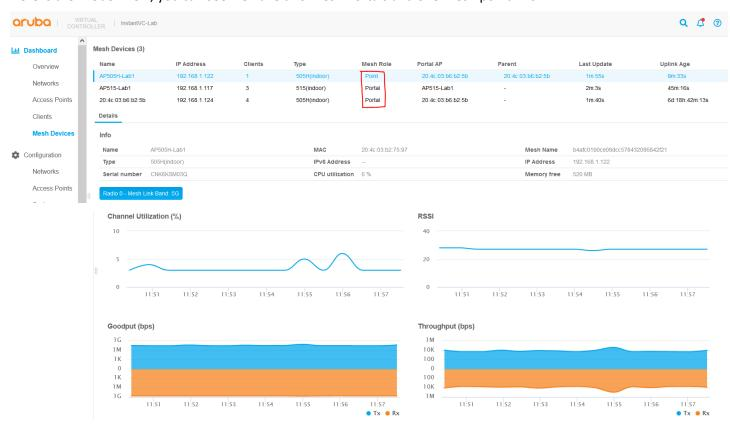
We see that the mesh link is on 5G radio. There are other mesh commands as well, like mesh cluster topology. These commands are run on the Virtual controller (VC).
