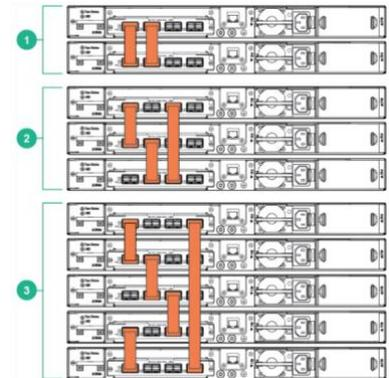
For the 3810M, the recommended topology for stacks of up to 5 members is a *mesh*; each stack member is connected to every other member to maximize reliability by providing multiple paths for rerouting traffic in the event of a link or chassis failure. For stacks of greater than 5 members, the ring topology, as described above, is recommended.
