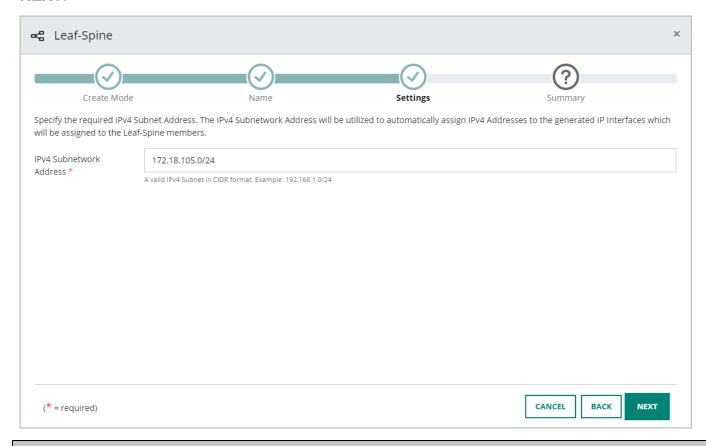
Use a subnet that is distinct from the subnets you plan to use in your overlay networks. The provided subnet will be used to configure routed ports on the fabric switches. In order to simplify route summarization between the campus and data center, ensure this range is unique to the underlay.
