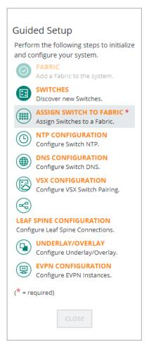
**Step 2:** Assign switches to the fabric grouped by role. Use the drop-down to expand a list of switches and roles available. For a large fabric the form can be used to filter on hostname. First select all spine switches, select **Spine** as Role, and then click **ADD**.
