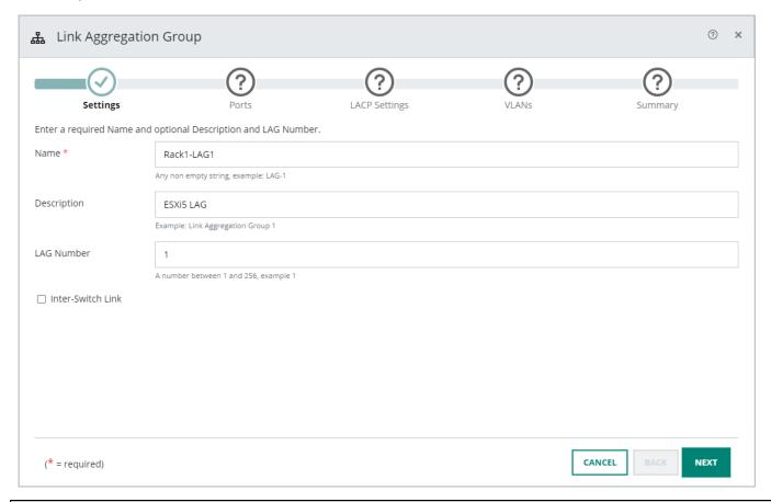
Consider using a **Name** and **LAG Number** which will help to identify the hosts where they are connected.
