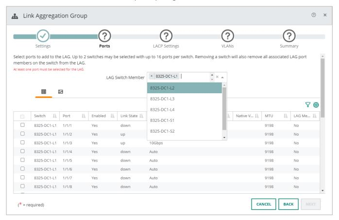
**Step 5:** From the Link Aggregation Group Ports page, change to **Switch View** mode to make it easier to identify the ports.
