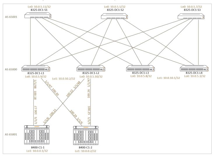
When using MP-BGP with EVPN address families, type-2 EVPN routes identify host reachability while type-5 routes identify network reachability inside the data center. EVPN host routes should be summarized when propagated outside of the data center. When combining multiple overlay VRFs into a single IGP and/or BGP network the use of Inter-VRF Route Forwarding (IVRF) is required. This allows routes to dynamically propagate from data center overlay VRFs into a common external VRF.
