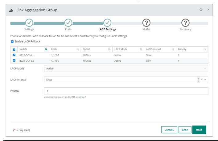
Aruba CX switches default to Active to ensure that LACP can be established regardless of the LACP configuration of the host platform. The default settings are recommended.
