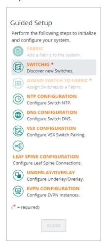
**Step 2:** From the Discover Switches page, enter the OOBM IP information for the fabric switches. Switch IP addresses can be entered in a comma separated list or in one or more ranges.
