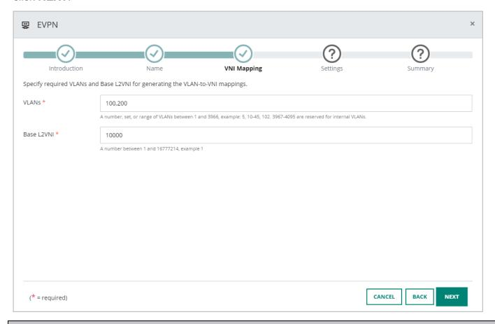
The Base L2VNI value which will be the base for automatically generated VNIs.
