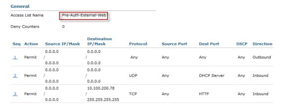
The ACL gives access to the website on Aruba Clearpass and DHCP. DNS is allowed by the WLC.
