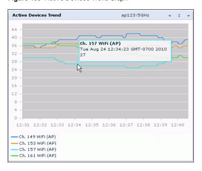
An Active Devices Trend chart created by a hybrid AP displays data for the single channel monitored by that device. For spectrum monitors, the Active Devices Trend chart can display values for up to five different channels and device types. These graphs show the following data by default:
