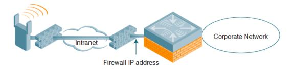
In any of the described deployment scenarios, the IPSec VPN tunnel can be terminated on a local, with a master controller located elsewhere in the corporate network (Figure 68). The remote AP must be able to communicate with the master controller after the IPSec tunnel is established. Make sure that the L2TP IP pool configured on the local controller (from which the remote AP obtains its address) is reachable in the controller network by the master controller.
