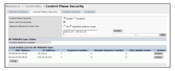
If your deployment includes both master and local controllers, then the campus AP whitelist on every controller contains an entry for every secure AP on the network, regardless of the controller to which it is connected. The master controller also maintains a whitelist of local controllers using control plane security. When you change a campus AP whitelist on any controller, that controller contacts the other connected controllers to notify them of the change.
