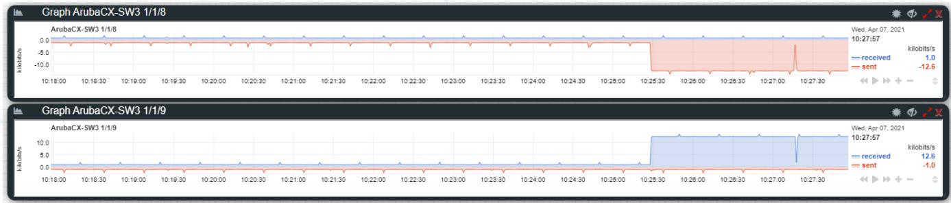
The egress port being loaded on SW3 is determined by the hashing algorithm on SW3, whereas the ingress port being loaded on SW3 is determined by the hashing mechanism performed on egress direction from SW4. The VSX nodes will forward the traffic on the local VSX node in nominal situation, and will not use the ISL if all downstream switches are dual-attached to VSX primary and to VSX secondary.
