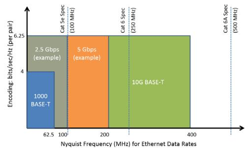
Figure 1. Relationship between cable category, frequency and Ethernet data rates - source: http://www.ieee802.org/3/cfi/1114\_1/CFI\_01\_1114.pdf Cabling in the field that is certified for 1000BASE-T operation has enough channel bandwidth to support 2.5 Gbps Smart Rate operation. While 2.5 Gbps operates at a higher frequency than 1000BASE-T (62.5 MHz), its coding, modulation, and error correction technique compensates for additional performance impairments.
