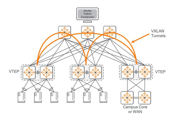
Attached hosts are learned at the leaf switch using Ethernet link layer protocols. Remote learning across the VXLAN fabric is accomplished using Multiprotocol BGP (MP-BGP) as the control plane protocol and a dedicated Ethernet Virtual Private Network (EVPN) address family for advertising host IP and MAC prefixes. This approach minimizes flooding while enabling efficient, dynamic discovery of remote hosts within the fabric.
