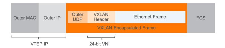
A VXLAN Tunnel End Point (VTEP) is the function within leaf switches that handles the origination and termination of point-to-point tunnels forming an overlay network. A single logical VTEP is implemented when redundant leaf switches are deployed in a rack. Spine switches provide IP transport for the overlay tunnels, but do not participate in the encapsulation/de-encapsulation of VXLAN traffic.
