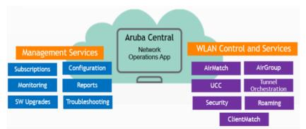
As you can see in the above diagram, the classic components that would normally run on mobility master or instant APs are now run as services in Aruba Central. I am talking about AirMatch, Roaming, ClientMatch, etc.
