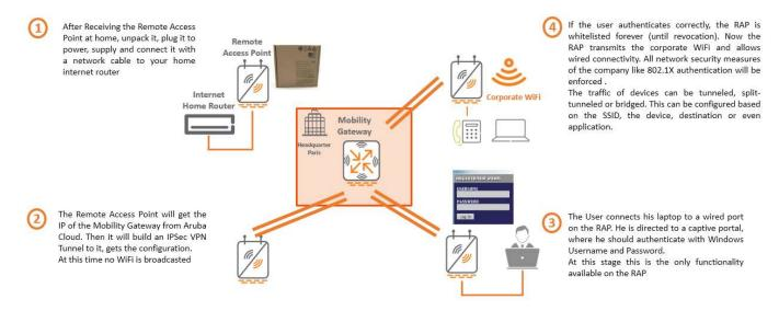
As seen in the figure, the key element here is that the RAP allows no wired or wireless connectivity until the user connects his laptop to a wired port on the RAP and authenticates on the captive portal using his Active Directory or Windows username and password. The user does it once; after that the RAP is whitelisted and will allow the configured settings like WiFi and Wired connectivity. This step prevents the RAP from coming under unauthorized hands before it reaches its destination.
