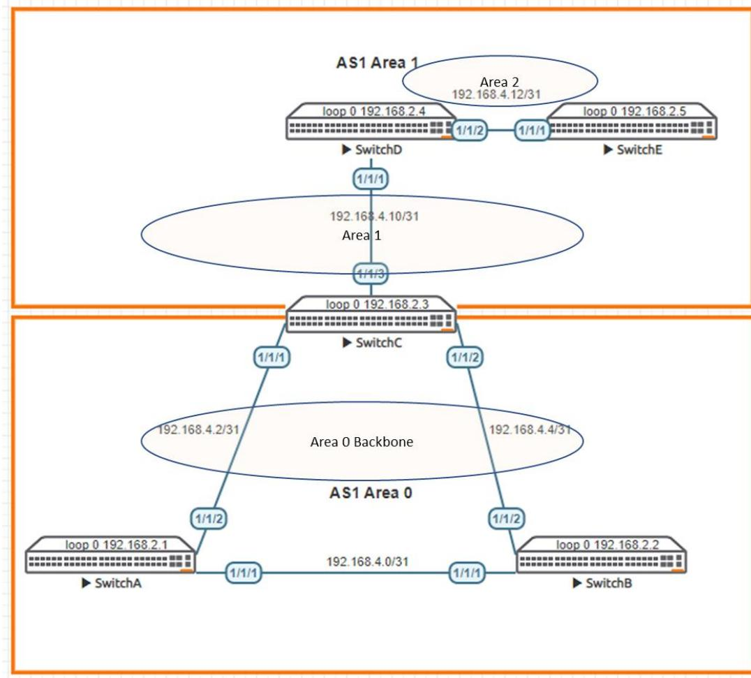
Configure Switches A to E with their appropriate configurations. OSPF routing area configurations are presented with their full notation but can be abbreviated; as in area 0.0.0.0 to area 0 and area 0.0.0.1 to area 1
