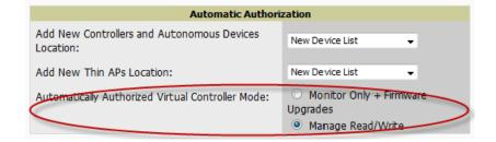
When the second Instant contacts AirWave using the DHCP server options as described previously, and that second Instant device has the same Shared key, it shows up on AirWave as shown below. Because the devices are in **Manage Read/Write** mode, there is no need for manual intervention to provision these new
