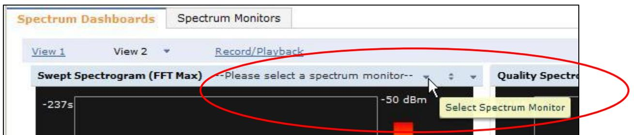
Here the pull down was used to select the AP set as the spectrum analyzer. In this example AP name 00:24:6c:c9:2d:c3 is selected to display the 2.4GHz band.
