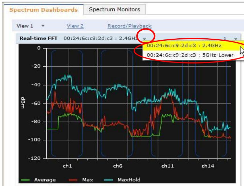
Note that other menu options are available to change the spectrum display. The display selected below is showing "Real Time FFT" per 2.4GHz band channel.
