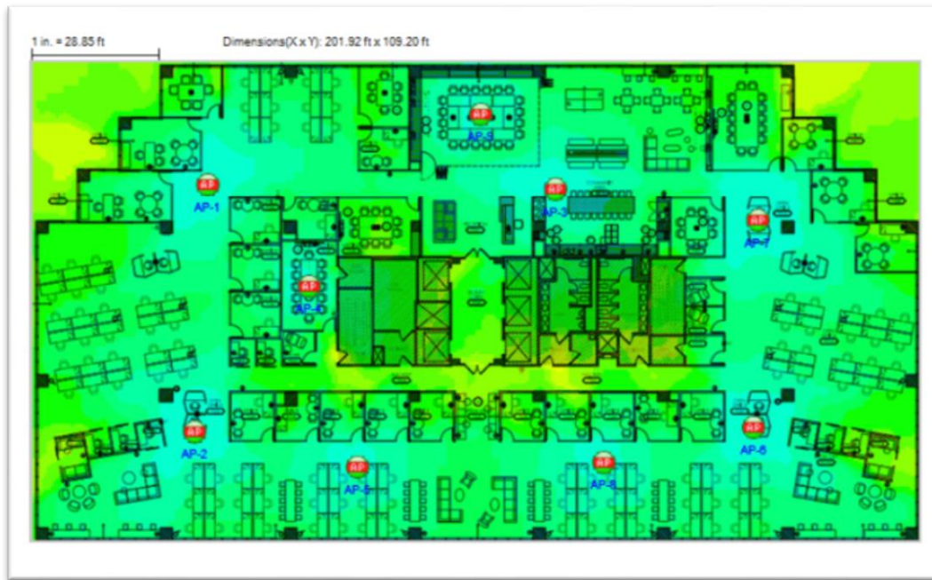
Figure 1 A floorplan showing complete RF coverage from a number of APs
